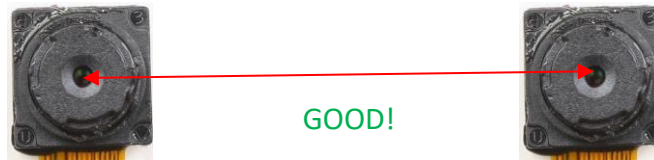
Figure 31- Good example of camera placement
