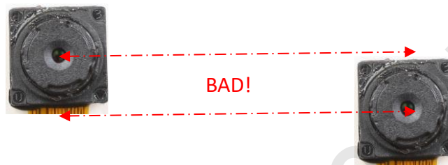
Figure 32- Bad example of camera placement.
